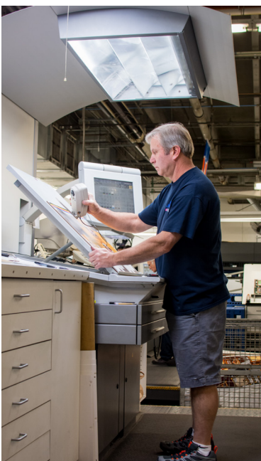
Robert Leeper, lead pressman on Warneke Paper Box's Heidelberg Speedmaster CD 74, checks the color density on a printed sheet.
